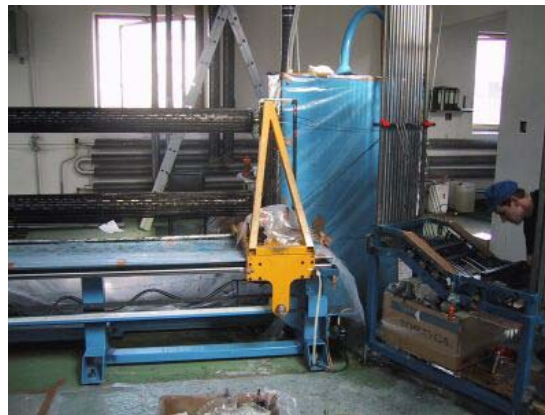
Fig. 2: Winding machine developed in the Compo Tech PLUS Ltd. Company.
