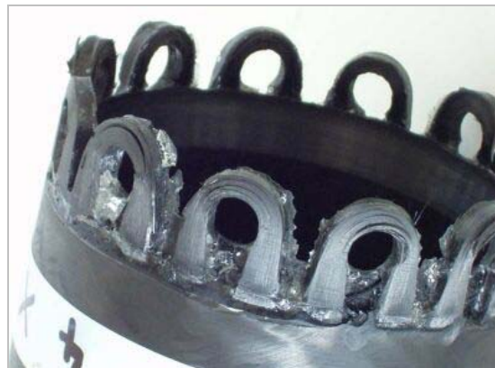
Fig 4: Integrated wound in "pin joint", Compo Tech hydraulic cylinder sample, after break test.
